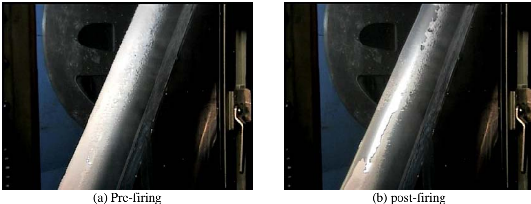
Figure 4: Typical EMEDS performance on 0.040" aluminum skin (200 mph, 13°F, 0.7 g/m 3 , 20 microns)
