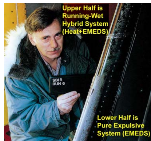
Figure 6: Hybrid system (running-wet anti-icing on LE and EMEDS expulsive deicing downstream)
