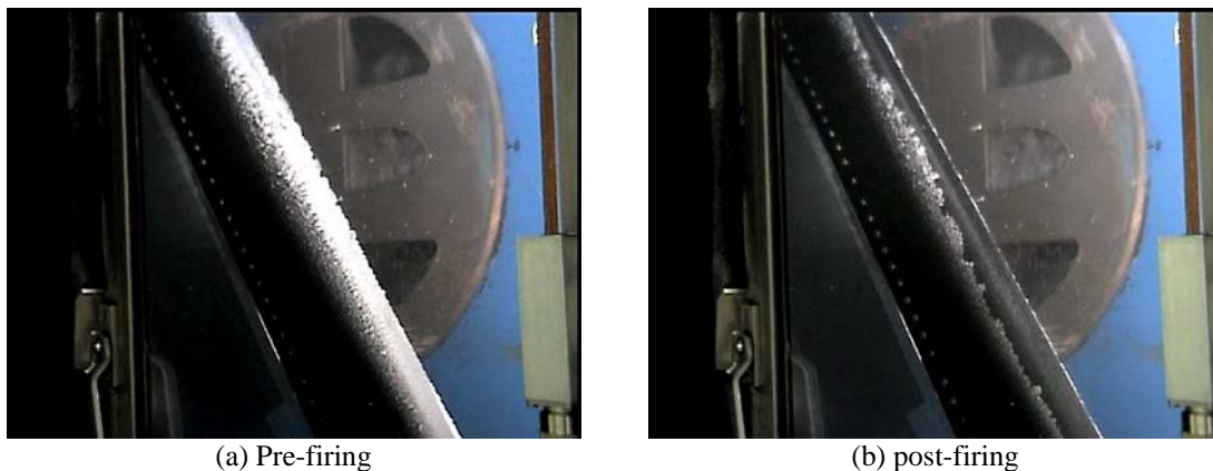
Figure 5: Typical EMEDS performance on painted 0.025" aluminum skin (same conditions as above)
