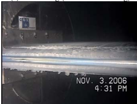
(c) Pre-deicing (44 minutes in icing)
